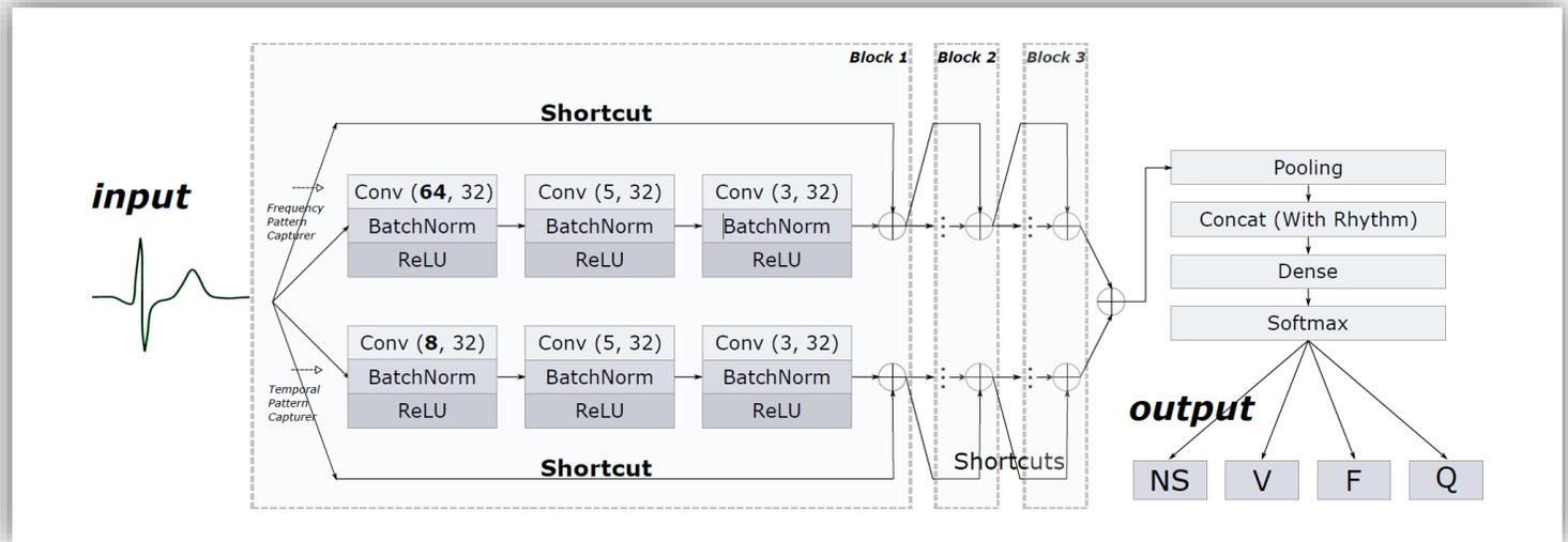
1. DDCNN accepts segmented heartbeats as input and outputs a prediction of probabilities of the N&S-bundle, V, F and Q classes.
